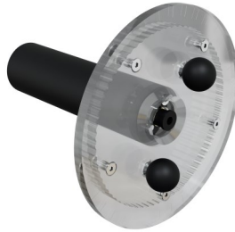
Tapped cylinder attached to circular protractor (Worksheet 2)
