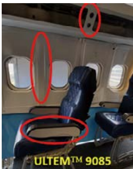
Diversified Functional & Engineering parts (Incl. thermo, flame, smoke, toxic-resistant plastic) 多樣化功能及工程部件 (包括耐高溫、防火、煙、毒物料)
