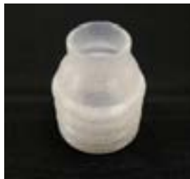
Silicone FAM Printer Materials: Silicone (3rd Party materials, Shore A: 30, 50, 65, 70)
