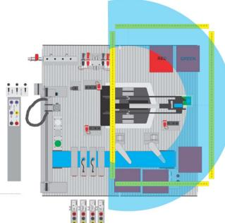
Students create a counter sorting program in which the Robot Arm will collect plastic counters and using the colour sensor, they are sorted into appropriate collection bins. The system can be operated manually or using internet communications, students can implement a handshaking system to automate the process.
