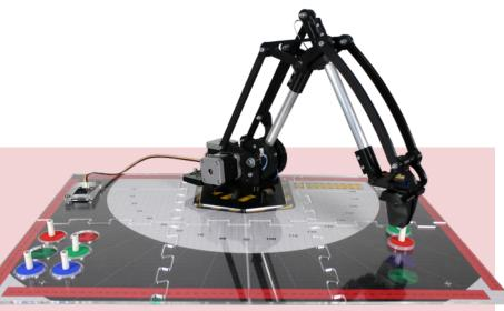
With base, shoulder and elbow rotation and functional gripper, the arm itself delivers fast, accurate and repeatable movement. The stepper motor driven arm delivers an accuracy to 0.04 degrees per step, < 0.5mm XYZ. The kit is supplied with a number of coloured counters which can be moved by the arm into different locations in the work cell to study pick and place and sorting technology. It is also compatible with the Industry 4.0 Smart Factory (see pages 4 & 5).
